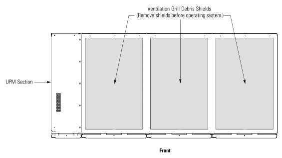
Figure 4-17. ISBM and UPM Section Debris Shields
